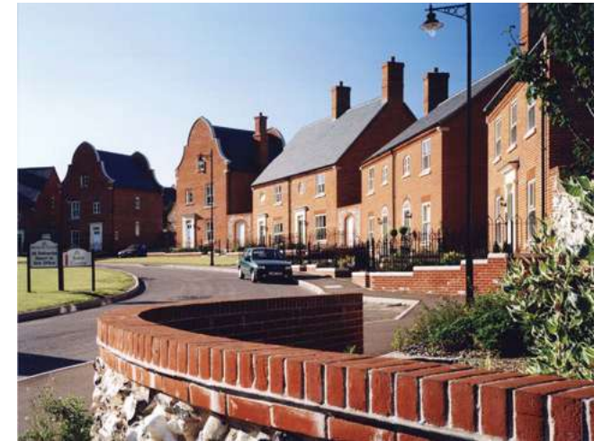
This neighbourhood in a semi-rural setting draws on local historical precedents to create a distinctive character. It is defined by the height and massing of buildings, variation in roof forms and material selection. Gables are paired to create a focal point and mark the entrance to a street. Trowse Newton, Norfolk.
